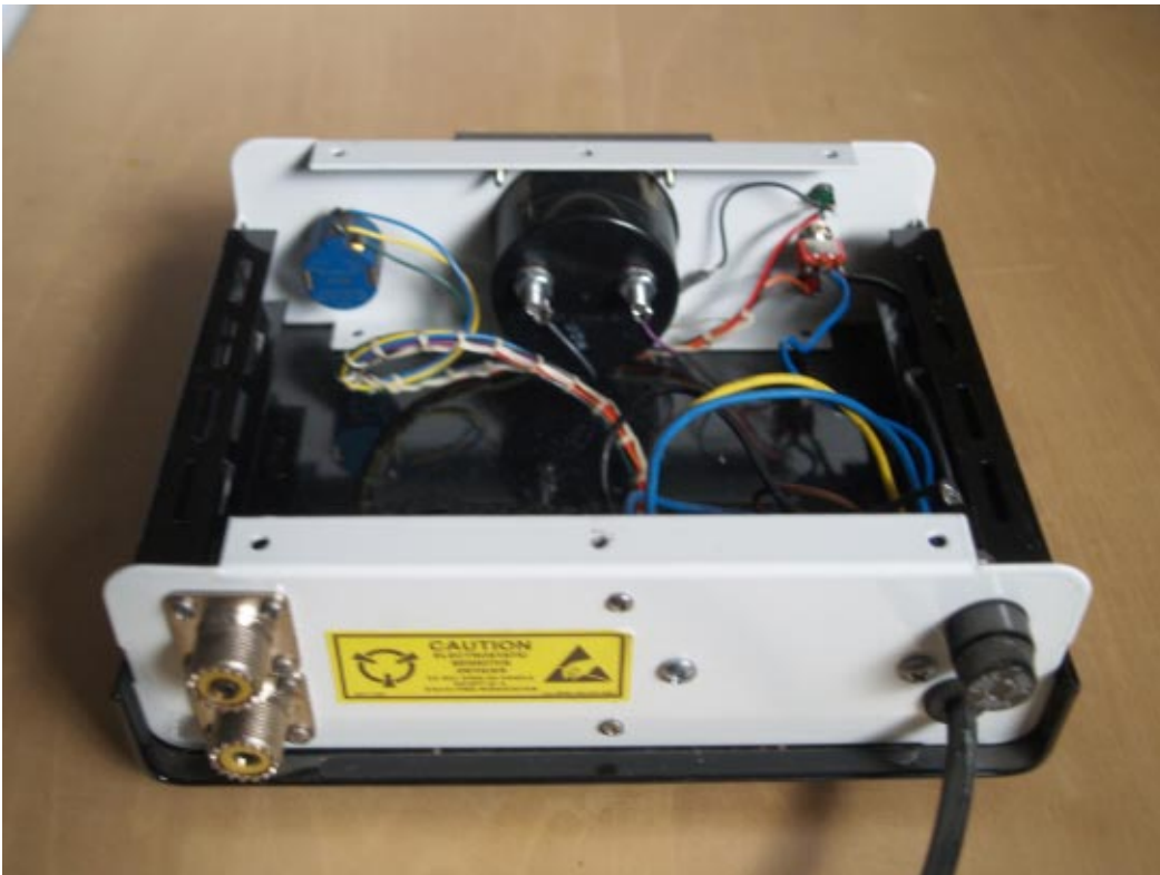
Fig. 14 - Active Antenna Power and Control Unit Prototype Front View (top) and Rear View (bottom)
