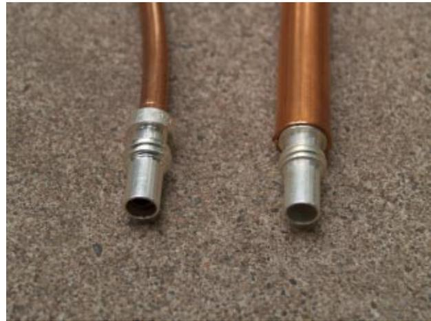
Fig. 11 - PL-259 Reducers Attached to 1/4" (left) and 1/2" (right) Copper Tubing
