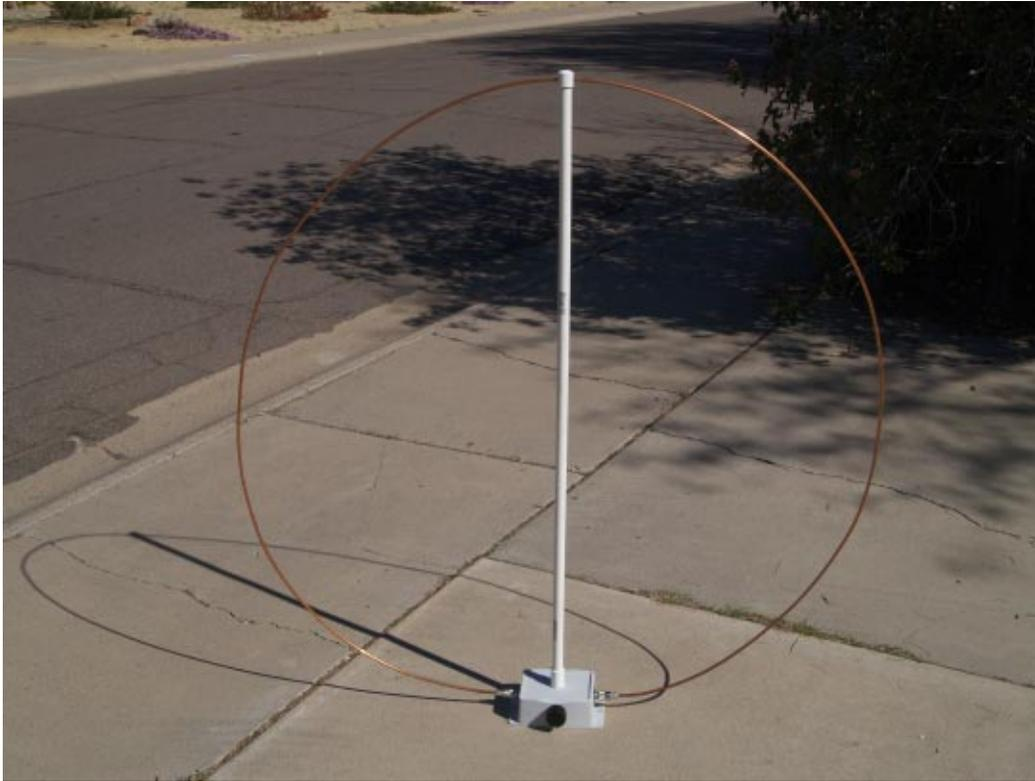
Fig. 14 - Fully Assembled Varactor-Tuned Indoor Loop Antenna
