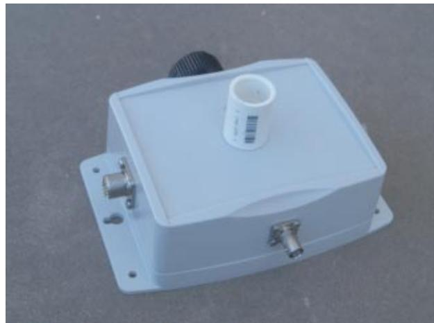
Fig. 10 - Varactor-Tuned Indoor Loop Antenna Base
