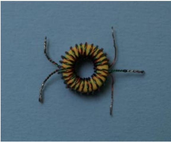
Fig. 5 - Construction Details for Transformer T1
