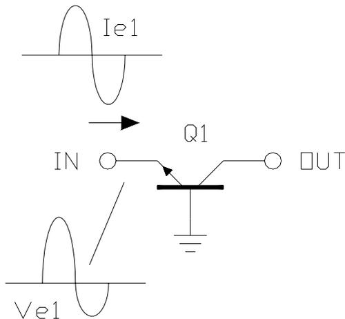
Fig. 1 - Common-Base Amplifier Input Characteristics
