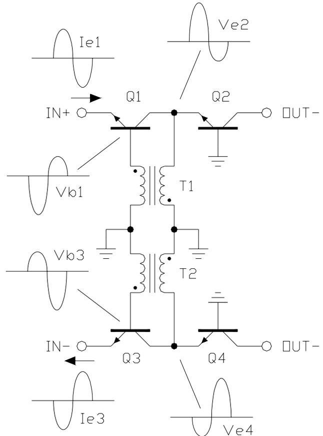
Fig. 4 - Balanced Common-Base Amplifier Using Cascade Linearization
