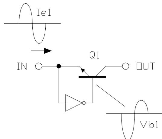
Fig. 2 - Basic Augmentation of the Common-Base Amplifier
