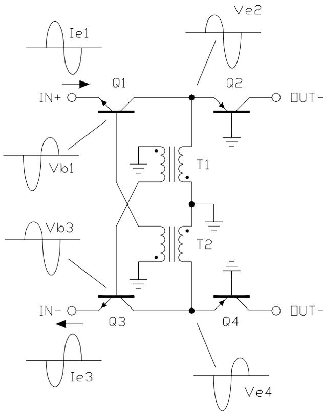
Fig. 5 - Linearized Common-Base Balanced Amplifier Using Linvill NIC Feedback
