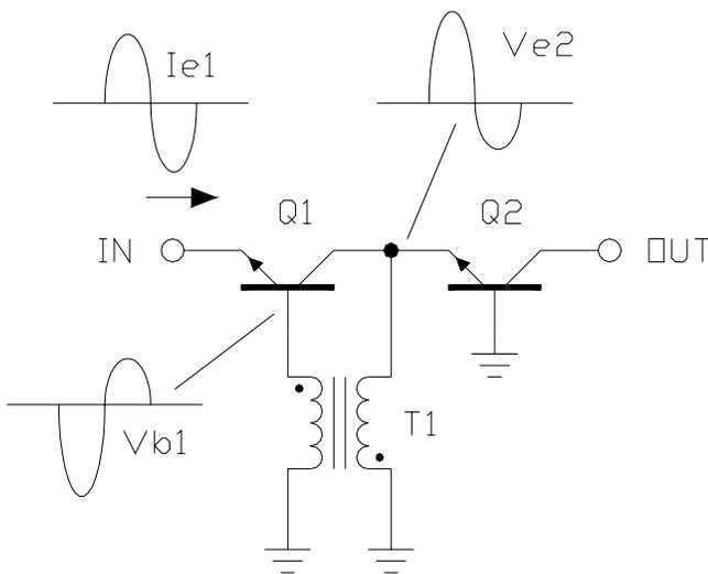
Fig. 3 - Cascade Linearization of the Common-Base Amplifier
