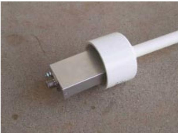
Figure 4 - Shielded Inner Housing:
