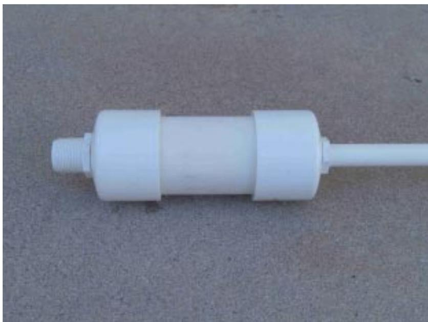
Figure 3 - Assembled Waterproof Outer Housing
