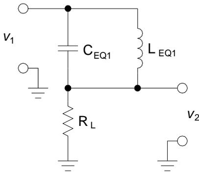
Fig. 10 - Equivalent Circuit for Measuring  $C_{EQ1}$
