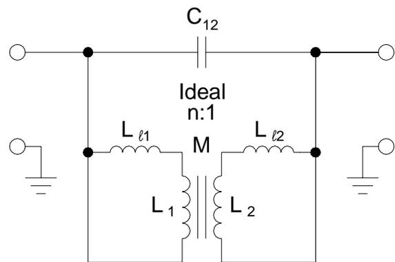
Fig. 8 - Circuit for Measuring  $C_{12}$
