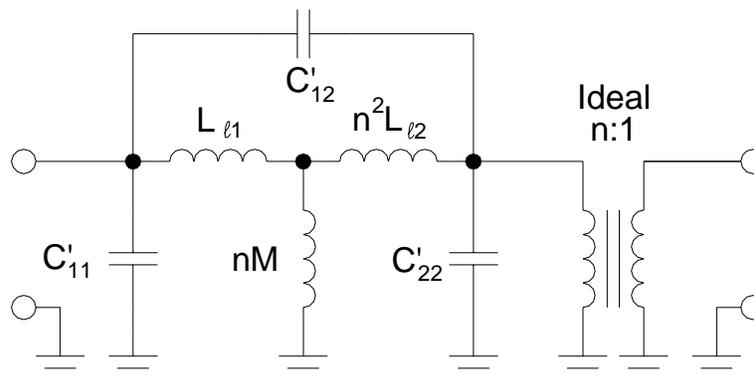
Fig. 4 - Complete Model of Lossless Wideband Transformer Referred to the Primary Side
