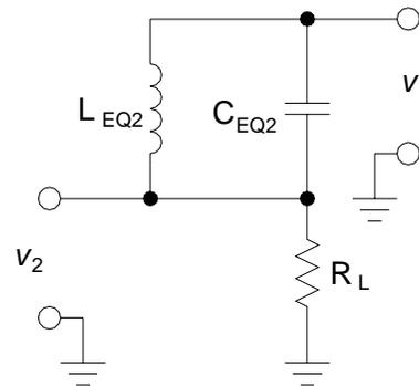
Fig. 12 - Equivalent Circuit for Measuring  $C_{EQ2}$
