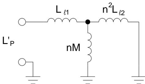
Fig. 6 - Equivalent Circuit for Measuring  $L'_p$
