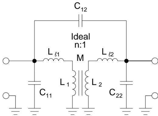
Fig. 3 - Complete Model of Lossless Wideband Transformer
