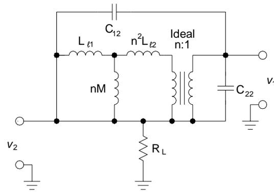
Fig. 11 - Circuit for Measuring  $C_{EQ2}$
