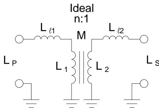
Fig. 2 - Circuit of 2-Winding Transformer Showing Winding and Leakage Inductances
