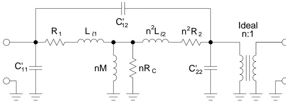
Fig. 5 - Complete Wideband Transformer Model
