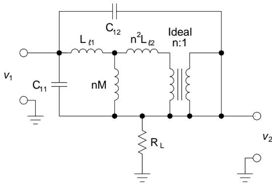
Fig. 9 - Circuit for Measuring  $C_{EQ1}$
