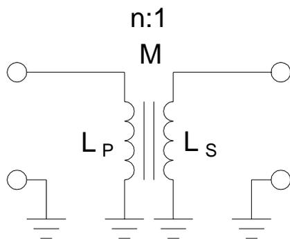
Fig. 1 - Circuit of 2-Winding Transformer
