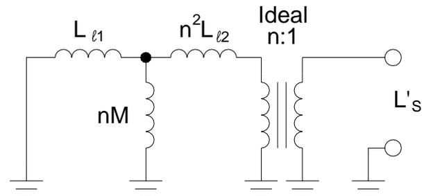
Fig. 7 - Equivalent Circuit for Measuring  $L'_s$
